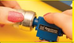
5. To unlock (when "Back Nut" is in unlocked mode) push the "Lock Nut" forward and stop reverse movement by setting your fingers onto the "Back Nut".
