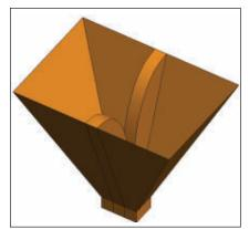
▲ Fig. 5 Dual-ridge horn model represented both the source antenna and calibration gain standard.
