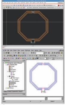
▲ Fig. 4 Layout of spiral inductor defined in Cadence Virtuoso imported into HFSS for 3D full-wave analysis.
