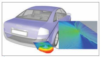
▲ Fig. 1 77 GHz radar antenna: electric near field, far field at 77 GHz.
