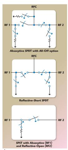
Fig. 3 Basic switch architectures that describe the behavior of the unused switch port.
