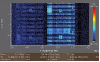
▲ Fig. 1 High Resolution Spectrogram Full of two LTE channels (resolution 8 µs) showing the frame structure with its resource grid and synchronization signals.
