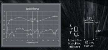
Marki Microwave offers accurate simulation models for all new Microlithic mixers. These models can predict isolations and spurious products.
