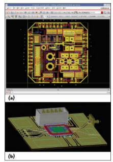
Fig. 1 EM simulation of parts of the RFIC together with the QFN package and the board.
