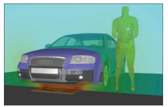
▲ Fig. 2 Wireless charging system: E-field at 1 MHz, averaged induced in body electric field at 90 kHz.
