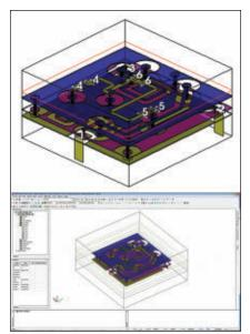
▲ Fig. 5 Layout of structure with defined ports originally designed in AWR imported into HFSS for 3D full-wave analysis.
