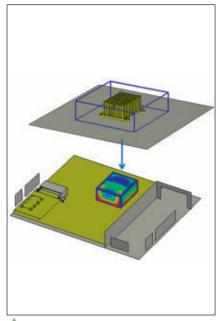
Fig. 9 A nearfield source representing a heatsink in an EMC simulation of a router.
