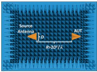
tenna and  $\lambda$  denotes  $\triangle$  Fig. 1 Measurement configuration for the gain-transfer method
