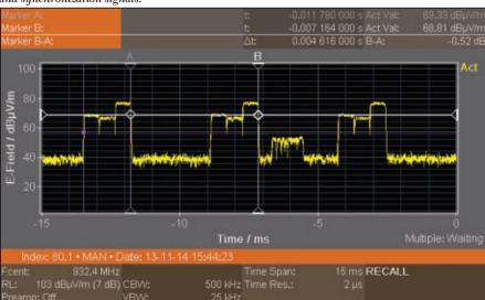
$\triangle$  Fig. 2 A GSM downlink signal triggered on the rising edge (time resolution 2  $\mu$ s) showing the 546  $\mu$ s timeslots (frame duration is measured using markers A and B:  $\Delta t = 4.616$  ms).
