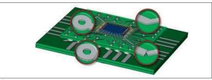
▲ Fig. 8 An imported model of a package, showing the automatic cleaning of faceted edges and healing of shape errors.
