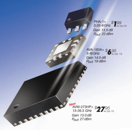
*Mini-Circuits' New AVM-273HP+* wideband, 13 dB gain, unconditionally stable microwave amplifier supports applications from 13 to 26.5 GHz with 0.5W power handling! Gain flatness of  $\pm 1.0$  dB and 58 dB isolation make this tiny unit an outstanding buffer amplifier in P2P radios, military EW and radar, DBS, VSAT, and more! Its integrated application circuit provides reverse voltage protection, voltage sequencing, and current stabilization, all in one tiny package!
