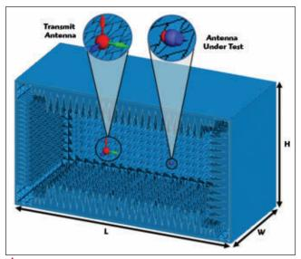
Fig. 2 Simulation configuration along with the dimensions for an anechoic chamber model.
