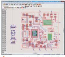
Fig. 4 PA module top-level test bench in ADS with look-alike symbol for the laminate.
