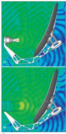
Fig. 10 Simulation of a reflector antenna with (a) a 3D model of the feed horn and (b) an equivalent nearfield source created with INSIGHT.
