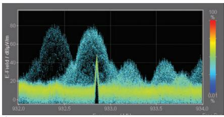
▲ Fig. 3 Persistence Spectrum of a GSM downlink signal showing underlying interference at around 932.8 MHz.
