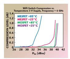
▲ Fig. 1 Compression characteristic of a MESFET versus a MOSFET WiFi switch showing the sharper compression behavior of the MOSFET device.
