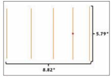
Fig. 6 Yagi-Uda model used for co-polarization antenna measurments.
