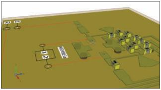
▲ Fig. 3 Amplifier design at 24 GHz.
