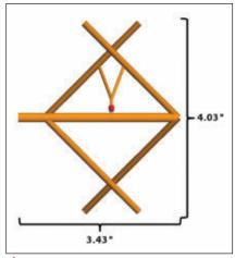
📤 Fig. 8 Shunt-fed slanted V-dipole model used for cross-polarization antenna measure-
