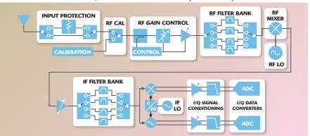
Fig. 4 Example receiver block diagram highlighting typical switching requirements.
