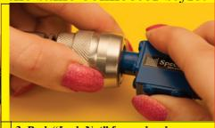
3. Push "Lock Nut" forward and engage the Push-On end of the Adapter with the mating female. Back nut must be released.
