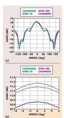
📤 Fig. 7 H-plane gain for a Yagi-Uda antenna, across all angles (a) and at broadside (b).
