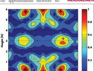
Fig. 4 Quiet zone error imposed by MoM/PO when operating at 500 MHz.
