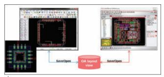
▲ Fig. 1 Advanced Design System 2014 uses the Open Access database, enabling bidirectional schematic interoperability with Cadence Virtuoso.
