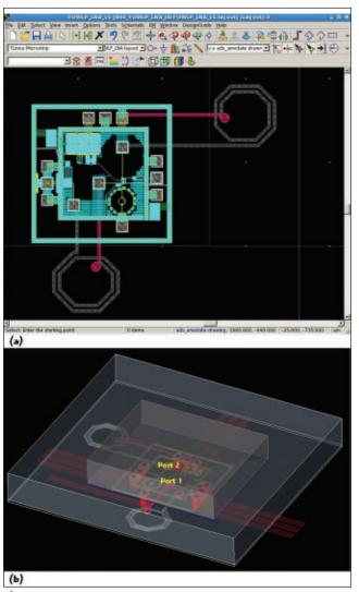
▲ Fig. 2 Fan-out wafer-level package test structure with integrated passives (a) and 3D view including solder balls and board traces (b).
